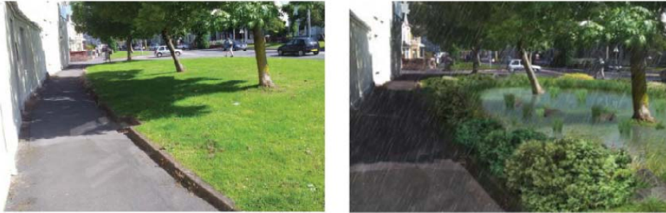
Figure 17 Example retrofit SuDS solution proposed for Gowerton and Llanelli
