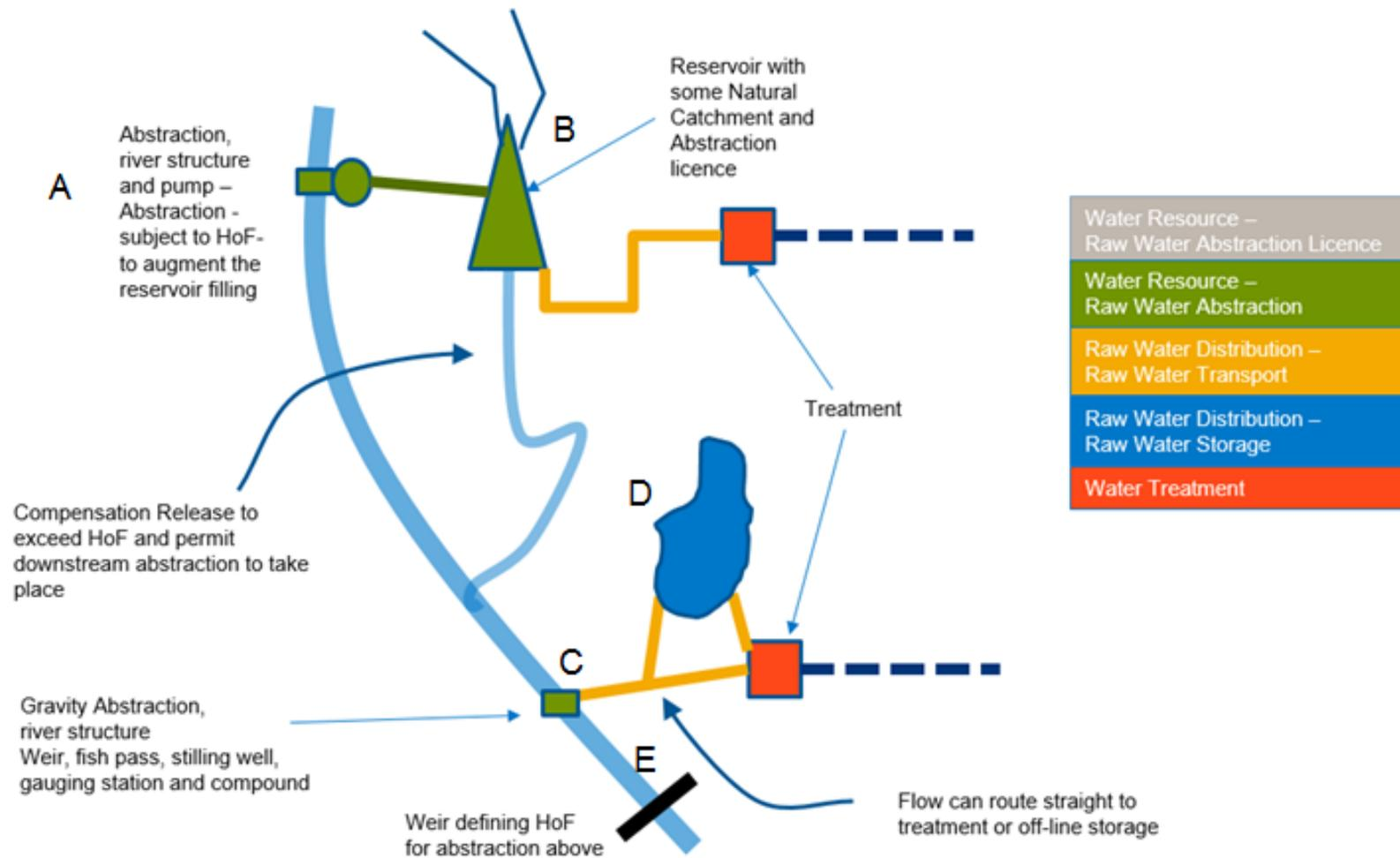
The above diagram shows a complex system based on achieving Hands off Flow (Hof) at a downstream Weir.
