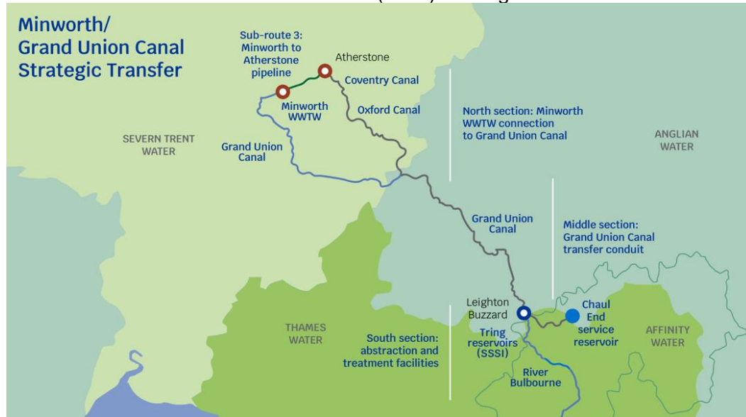
Figure 8 – Schematic of Grand Union Canal (GUC) Strategic Transfer from Minworth
