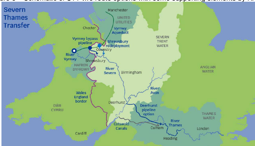
Figure 6 – Schematic of STT two route options with some supporting elements by RAPID
