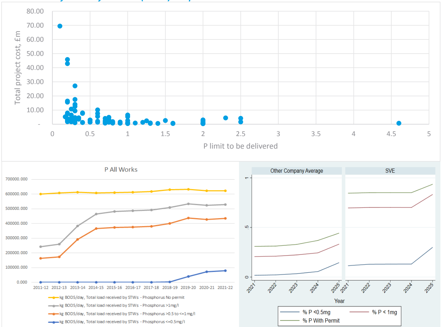
Figure 16: A collection of charts showing - Forecast project cost (£m) against p limit to be delivered (top) which shows tighter P consents incur significantly more cost; P consents rising across the industry (bottom left); and P Consents at Severn Trent against other companies, showing this is more of an issue for certain (inland) companies.
