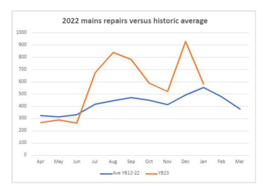
Whilst not the subject of this request, this comparison also highlights the impact of the prolonged period of high temperatures seen in the summer of 2022, driven by both the highest demand on record and the extreme impact on Soil Moisture Deficit experienced, which resulted in a material increase in mains bursts and associated water losses.
