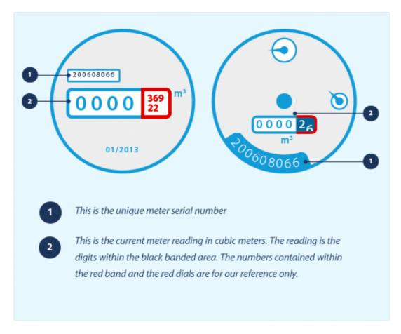
The black numbers register the cubic metres of water you've used. Red numbers record fractions of a cubic metre you've used. It's a good idea to keep an eye on your meter readings in case you spot anything unusual which may mean there's a leak somewhere. If you think you have a leak you can use the meter to check this.
