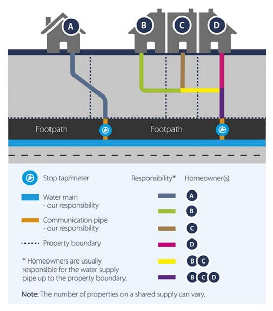
If the pipe is in poor condition, we recommend you and your neighbours replace it with separate pipes. This would improve both the flow and the pressure of water at your tap. We can require separation of a shared pipe in certain circumstances:
