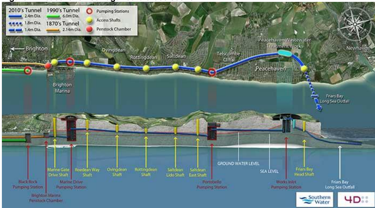
Figure 2: Peacehaven sewage route cross section
