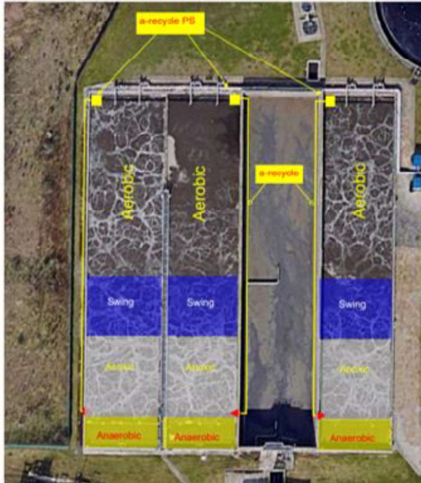
Figure 1.8 Biological Treatment Process Example
